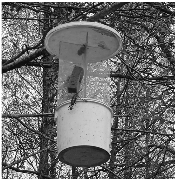
Figure 1. Bait-window trap (P. Ivinskis construction)
